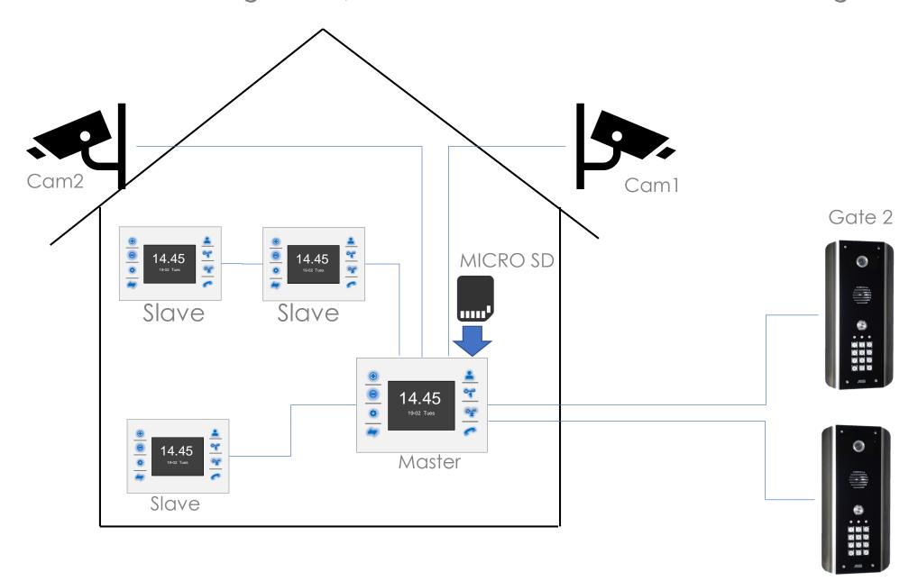
Monitor mounting Flush or Surface Recording 8Gb Micro SD card included, 32Gb Max Capacity Over 50 x 10 second clips (200 on 32Gb card) Motion detection video algorithm Recording type **Recording channels** 1 (can choose to record from door, or camera) **Recording options** 10-60 second video, or still image Recording resolution 720 x 288 pixels 4.3 inch Screen size Scree resolution | 480 x 272
