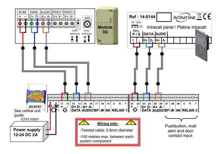
Intercom wiring to connectors 3 and 4 is the same when an extension board is used (12-0109).
