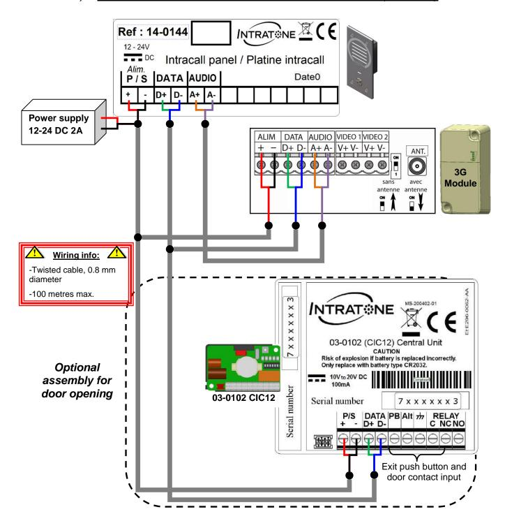
Up to three 12-0110 relay cards maximum can be added to this central unit to allow four doors to be opened together or separately.
