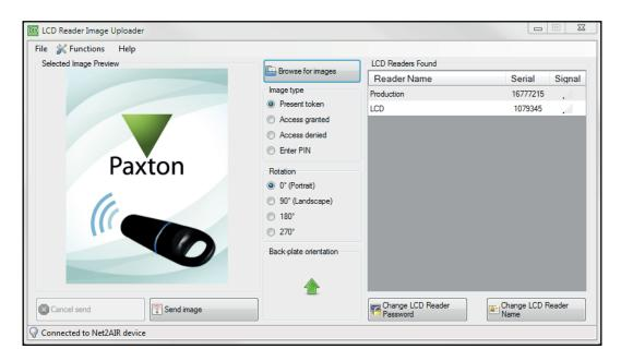
Close down any other Net2 applications, including the Net2 server, to avoid any USB program conflicts. Run the LCD reader image uploader and it will detect the USB Net2Air device connected to the PC. The PC will then detect and display any LCD units that are in range of the USB device.
