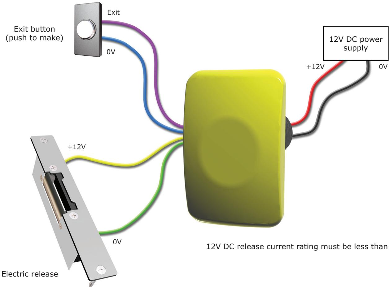
12V DC release current rating must be less than 1A.
