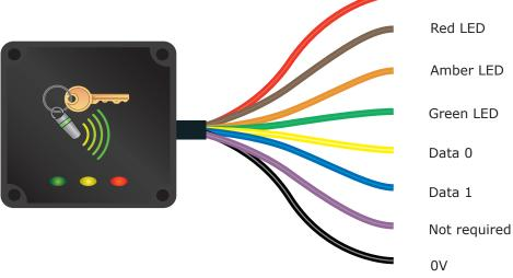
Pull directly to 0V to light LED
