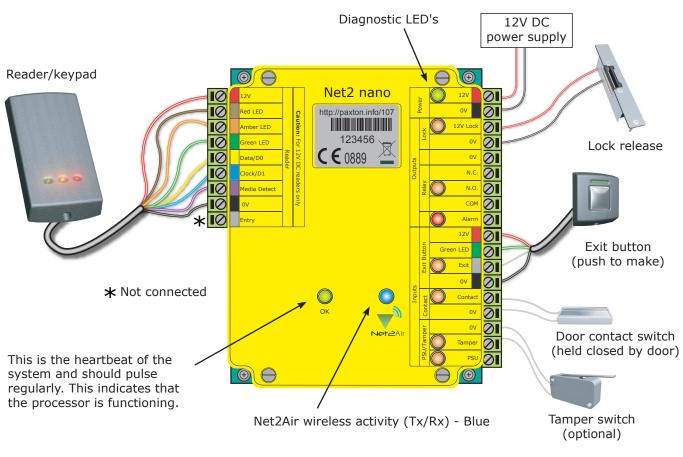
A new unit requires approximately 30 seconds after initial power up to self configure. During this time the OK LED will not be flashing.
