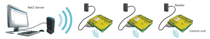
The reader's default indication has all the LED's on. Access granted is denoted with a single flashing Green LED. Access Denied is a single flashing Red LED.
