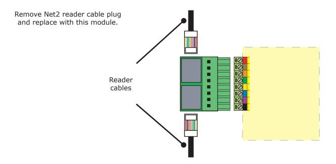
IMPORTANT: Ensure that only Paxton readers are connected to these RJ45 ports. Other equipment may be damaged if connected to these ports in error.
