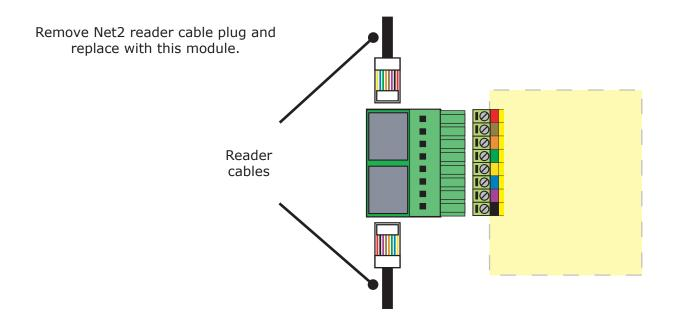
IMPORTANT: Ensure that only Paxton readers are connected to these RJ45 ports. Other equipment may be damaged if connected to these ports in error.
