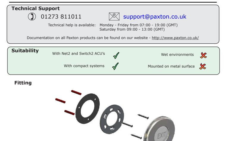
Fix the backplate to the wall with the stainless steel screws provided in the fitting kit. The small slot in the plate edge should be positioned at the bottom.
