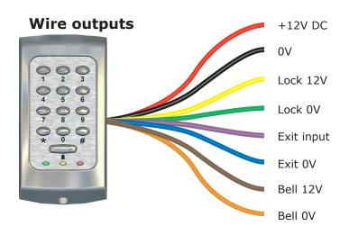
If the +12V bell wire (Brown) is not connected it must be terminated to avoid a short circuit.
