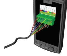
The unit should be mounted in conjunction with an electrical backbox to achieve the required clearance for the connector.
