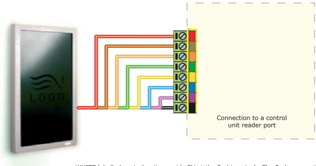
WHITE labelled control units provide 5V at the Red terminal. The Red power wire for the reader should therefore be directly connected to the 12V supply terminal.
