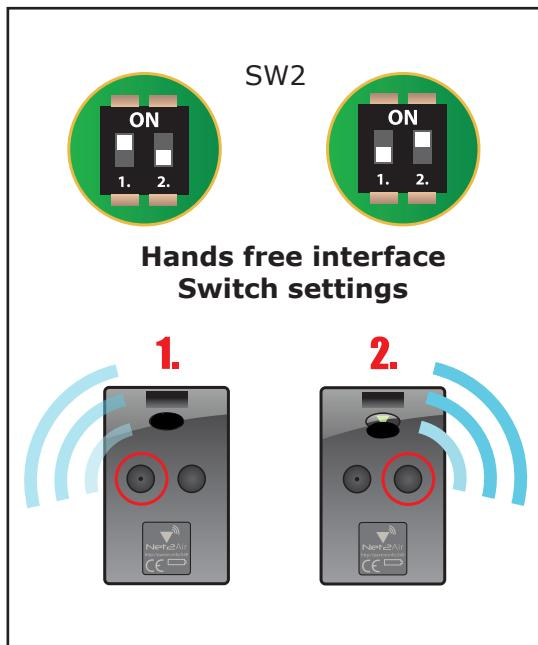
The hands free interface has a pair of switches labelled SW2. Select either switch 1 or 2 to set which button the interface will respond to.
