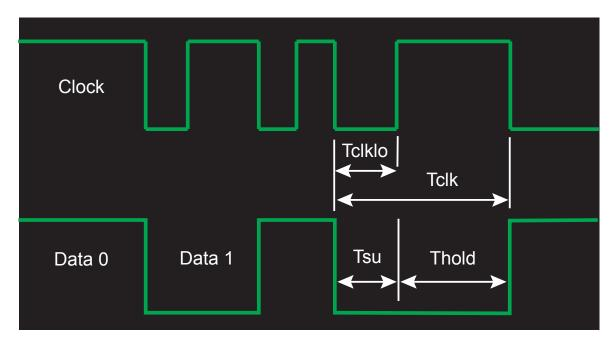
The Clock period (Tclk) is variable and will depend on the speed that the user card is swiped through the reader.
