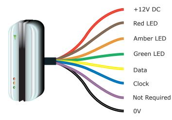
Pull directly to 0V to light LED Pull directly to 0V to light LED Pull directly to 0V to light LED Open collector Open collector
