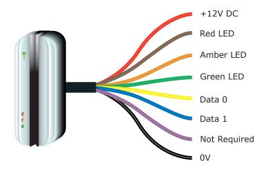
Readers can be extended using Belden CR9540 10-core overall screened cable to a maximum of 100 metres.
