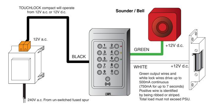
Duress codes can be programmed into the keypad. When a duress code is entered the lock output will activate for the door open time and the bell output will be activated for 30 seconds.
