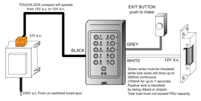
An internal push-to-make button can be used where electronic exit is required. When the button is pressed the doors electric release is activated. Any number of exit buttons can be fitted.
