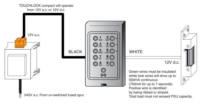
If the correct code is typed in the release is powered and the door unlocks.
