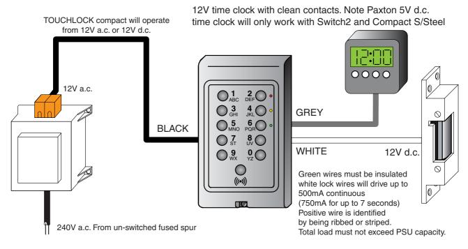
Where a door needs to be held open automatically a time clock can be wired into the keypad as shown above. The voltage free contact outputs from the time clock would be connected to the grey wires of the keypad. A standard central heating timer can be used.
