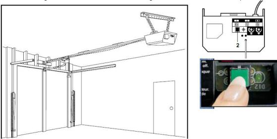
To delete all remote control codes. Press & hold the Green button until the Green LED goes out, then let go. (Approximately 9 seconds).
