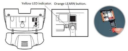
3. Press & hold your chosen button on the remote control, for 3 seconds, and the LEDs light will flash. Now let go of the remote control button, LED goes out, and the remote is ready to use.
