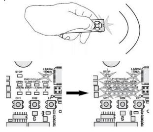
To delete all remote control codes. Press & hold the CH1 button until the red LED goes out, then let go. (Approximately 25 seconds).
