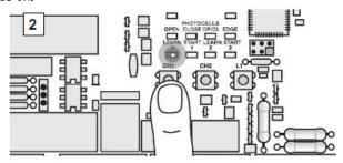
3. Press & hold the top button on the remote control, for 3 seconds, and the LEDs light will flash. Now let go of the remote control button, LEDs will goes out and then back on again, and the remote is ready to use.
