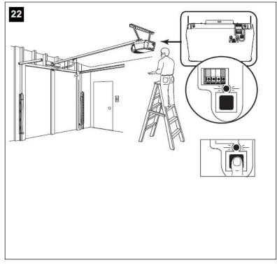
To delete all remote control codes. Press & hold the orange button until the orange LED goes out, then let go. (Approximately 9 seconds).
