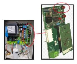
3. Press & hold the top button on the remote, for 3 seconds, and the LEDs will flash. Now let go of the remote button, LEDs will goes out and the remote is ready to use.
