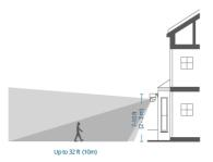
To ensure that no detection is missed, do not install the camera directly facing the monitoring area. Instead, maintain an angle to avoid any potential blind spots.
