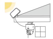
1. Drill holes with a 15/64 inch (5.95 mm) drill bit with the provided positioning card, then insert the anchors into the holes.
