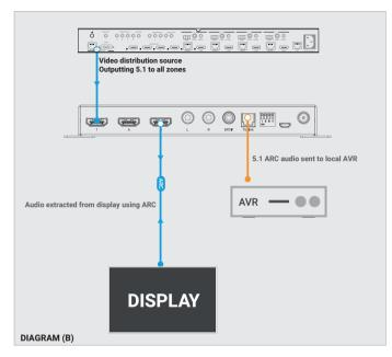
In diagram (B) the source content is being provided by a video distribution system like MHUB PRO (4x4) 40, here, it is presumed that all outputs from MHUB are delivering 5.1 audio. This is being fed in to and passed through the Dolby Digital Down-Mixer to the display. Using ARC it is now possible to extract the 5.1 audio back to the Dolby Digital Down-Mixer and route it to a local AVR using the Toslink port.
