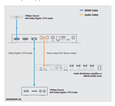
In diagram (A) an 18Gbps source outputting a digital audio format such as Dolby Digital or DTS is fed in to the input port on the Dolby Digital Down-Mixer. The audio is down-mixed to 2Ch stereo internally and extracted from the analogue audio ports which then is fed to an audio distribution amplifier or MHUB AUDIO (6x4) for distribution around a property. Simultaneously, the AVR receives an untouched HDMI signal and output whatever the source device is sending.
