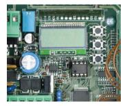
Built-in receiver, integrated into the controller, programmable via LCD display.
