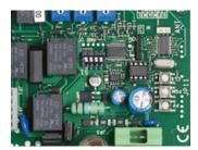
Built-in receiver, integrated into the controller, programmable via dip-switches/trimmers.
