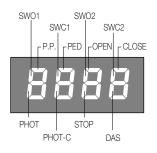
One segment of the display is linked to each input. In the event of failure it switches on according to the following scheme.
