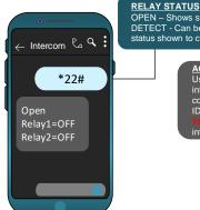
OPEN – Shows status of the input terminals called DETECT - Can be used with a limit switch. Relay status shown to check if any relay is latched.
