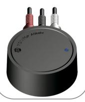
6. If connection failed, LED will flash blue until it goes into standby.
