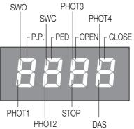
The Normally Closed (N.C.) inputs are represented by vertical segments. The Normally Open (N.O.) inputs are represented by horizontal segments.
