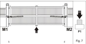
The gate stops and motor M1 starts an opening cycle. Press agin P1 in the point where you desire to set the leaf delay in opening.
