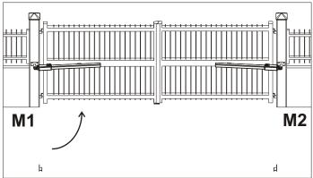
At this point if the gate doesn't reach the mechanical stop in opening, increase trimmer Rv4 (rotate clockwise) and give again a START impulse.
