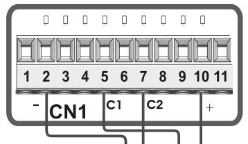
THIS SCHEME IS AN EXPAMPLE FOR HOW TO CONNECT EVENTUAL MAGNETIC LOOPS.
