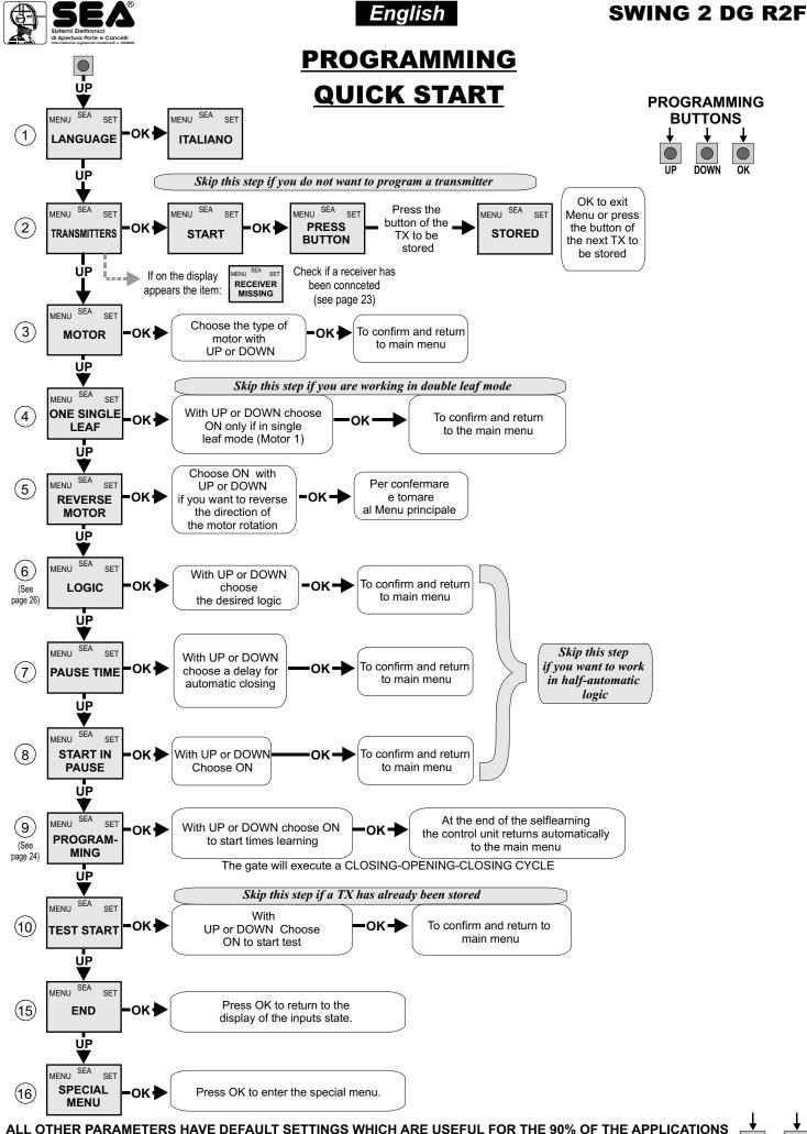
ALL OTHER PARAMETERS HAVE DEFAULT SETTINGS WHICH ARE USEFUL FOR THE 90% OF THE APPLICATIONS BUT CAN BE HOWEVER SET THROUGH THE SPECIAL MENU. FOR ENTERING INTO THE SPECIAL MENU MOVE ON ONE OF THE MENU AND PRESS THE UP AND DOWN BUTTONS AT THE SAME TIME FOR 5 S.
