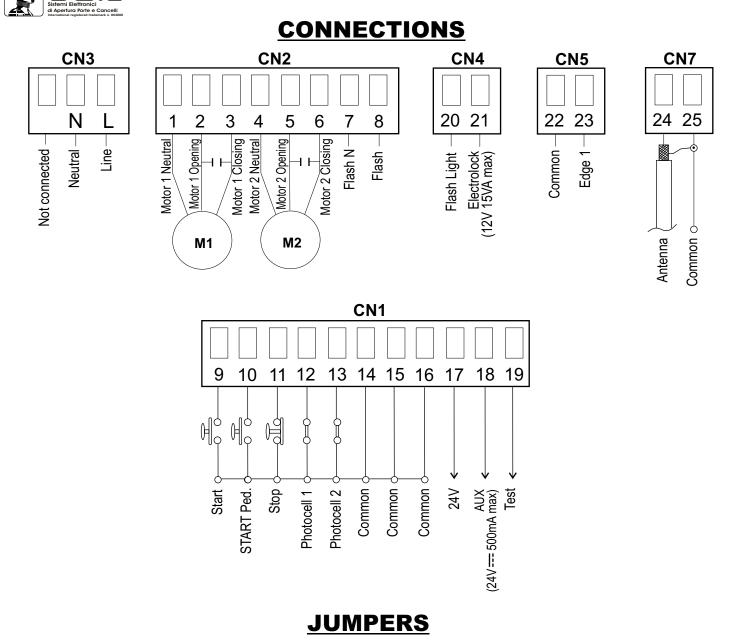
WARNING: The control unit is designed with the automatic detection of not used N.C. inputs (Photocells and Stop) except the SAFETY EDGE input. The exclude inputs in self-programming can be restored in the "Check inputs" menu without need to repeat the programming (page 36).
