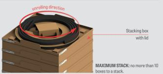
ASO edge material for self-assembly MUST be stored in a cool, dry environment away from sources of water or heavy contaminants. Before attempting to assemble contact edges the material should be checked thoroughly for moisture or contaminants and cleaned and dried appropriately.
