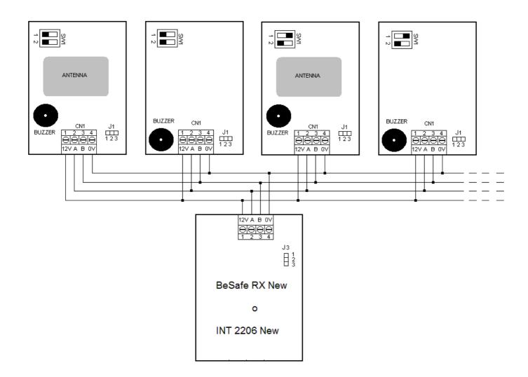
It is possible to connect to every single BeSafe RX New receiver or Interface INT 2206 NEW up to 2 BeSafe Reader NFC devices. By dip switch SW1 in advance you must assign to each BeSafe Reader NFC its own address:
