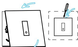
Attach your iotty Light Switch faceplate starting from the upper or the lower side.
