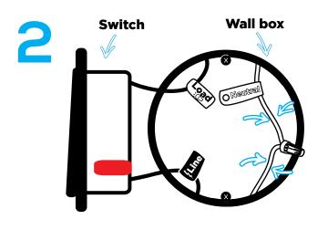
Unscrew and disconnect the wires from the old switch using a screw driver.
