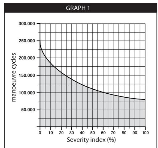
The durability values specified in the graph are only obtainable if the maintenance schedule is strictly observed (Chapter 7). The lifetime is estimated on the basis of design calculations and the results of tests performed on prototypes. Being only an estimate, it does not constitute any form of guarantee on the actual lifespan of the product.
