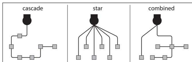
02. Observe Fig. 3 to understand how to position the electrical cables in the environment (it is advisable to draw on paper a similar layout, adapting it to the relevant requirements).
