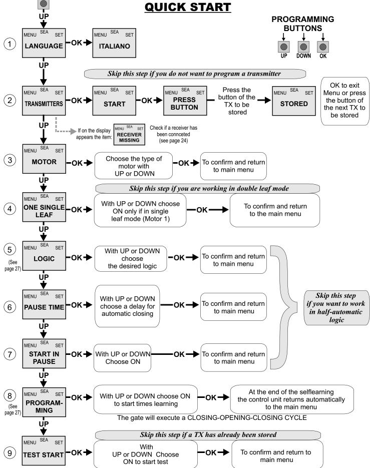
ALL OTHER PARAMETERS HAVE DEFAULT SETTINGS WHICH ARE USEFUL FOR THE 90% OF THE APPLICATIONS BUT CAN BE HOWEVER SET THROUGH THE SPECIAL MENU. FOR ENTERING INTO THE SPECIAL MENU MOVE ON ONE OF THE MENU AND PRESS THE UP AND DOWN BUTTONS AT THE SAME TIME FOR 5 S. DOWN
