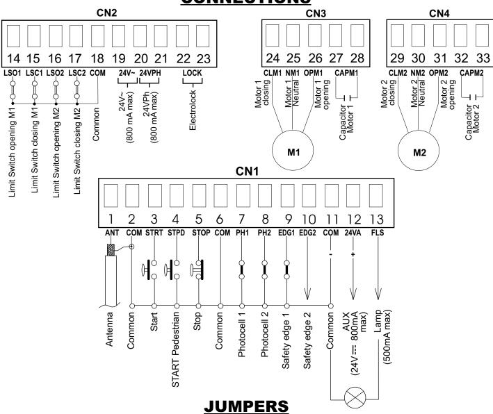
WARNING: The control unit is designed with the automatic detection of not used N.C. inputs (Photocells, Stop and Limit switch) except the SAFETY EDGE input. The exclude inputs in self-programming can be restored in the "Check inputs" menu without need to repeat the programming (page 38).
