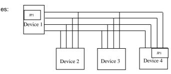
In the example above the jumpers should be placed on devices n. 1 and n. 4, irrespective of the type of device.
