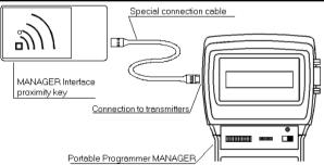
Insert one end of the special connection cable in the connection slot of the MANAGER+DCS Proximity Key Interface, and the other in the connection for transmitters of the Portable Programmer MANAGER+DCS (see figure page 6, no. 8 of the MANAGER+DCS manual).
