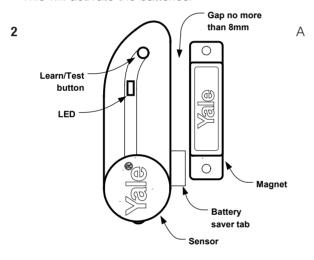
red light can be seen flashing through the lens. This will last for 30 seconds indicating the component's initiation.
