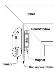
1 Find a location where the door/window contact is to be mounted. It should be mounted between the door/window frame and the door/window as shown at the top of the opening. The magnet is to go on the door/window while the sensor is to be placed on the frame. Windows can be protected in a similar way to doors. Make sure the tamper switch spring is fully depressed.
