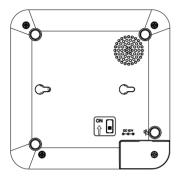
Unpack the kit content on a table. Remove the mounting plate (if fitted) from the control panel. Move rightwards to lock and move leftwards to release the panel (panel top facing the user). Connect the power adaptor.
