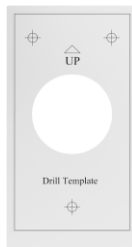
Drill Template for Intercom Panel (x1)
