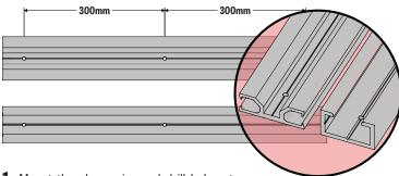
1. Mount the alu carrier and drill holes at points spaced 300-500mm apart minimum.
