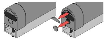
7. Finally ensure that water drains from the end caps have been removed as illustrated (for vertical installations remove only the lower water drain (for horizontal installations remove water drains from both ends of the safety edge) !WARNING! failure to remove water drains from the safety edge will invalidate any warranty.
