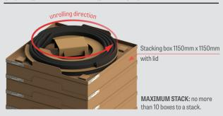
ASO edge material for self-assembly **MUST** be stored in a cool, dry environment away from sources of water or heavy contaminants. Before attempting to assemble contact edges the material should be checked thoroughly for moisture or contaminants and cleaned and dried appropriately.
