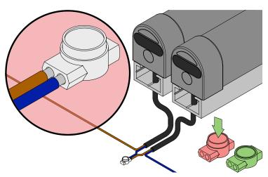
8. When joining cables between safety edges or junction boxes, be sure to use weather proof connectors such as gel crimps or properly soldered and heatshrinked connectors rated at IP 65 or above !WARNING! Failure to join cables properly will invalidate any warranty of the safety edge.
