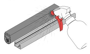
**4.** Use a soapy water spray solution to coat the rubber foot of the safety edge profile and the alu carrier before attempting to install the safety
