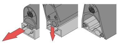
**5.** Fit the safety edge to the carrier as illustrated (edges with T foot slide in) (edges with a **C foot** clip in from above) (edges with a Clip foot, clip over from either side of the safety edge).
