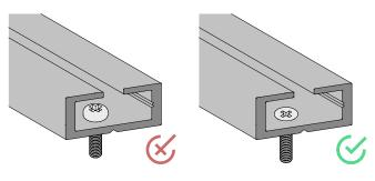
2. Use pan headed or counter sunk screws where possible to prevent snagging of the rubber edge profile on exposed screw heads.
