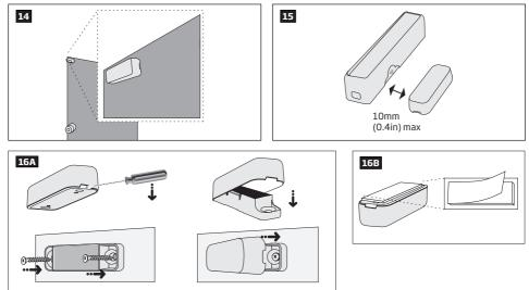
8. Remove the plastic tab inserted between one of the battery terminals and battery slots of EWD2.
