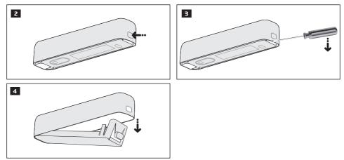
2. Remove the PCB (printed-circuit-board) from the enclosure.
