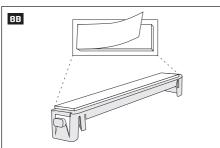
ATTENTION: When using this mounting method (fig. #8B), the back side of the enclosure will NOT be supervised by tamper switch.
