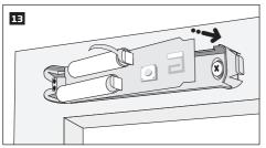
7. Open the magnet enclosure and screw in (see fig.#16A) or attach the magnet using double-sided adhesive tape (see fig.#16B) to the doors or window and ensure that the magnet is fixed at the same height as the EWD2 reed switch.
