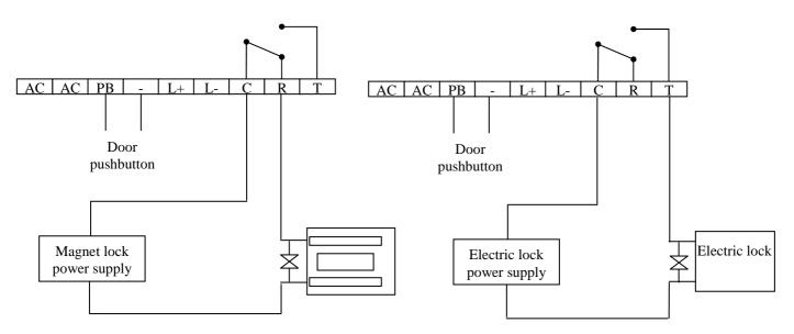
At rest, the magnet is powered and the door is locked. When the relay is activated by the central unit, the electric current releases the magnet lock (by pressing on a pushbutton or the use of an authorised badge).
