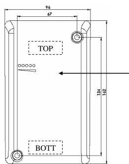
The GSM unit's LEDS show the GSM network reception quality around the installation:
