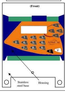
Stage 4: withdraw the central unit's housing, turn over the stainless steel base then insert the extension card's four clips into the four holes in the base.
