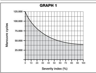
Example of durability calculation: \automation of a gate with a leaf length of 1.5 m with weight of 220 kg, for example, in a location subject to strong winds. Table 1 states the "severity index" values for this type of installation: 10% ("Leaf length"), 25% ("Leaf weight") e 15% ("Installation in windy areas").
