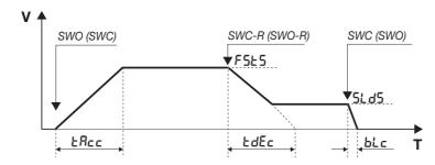
The V axis is the gate/door speed, T axis is the time required by the door/gate to move from a limit switch to the other. The parameters govern both the opening and the closing phases.
