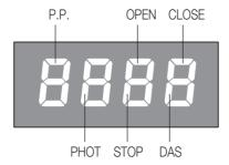
N.C. inputs are represented by the vertical segments. N.O. inputs are represented by the horizontal segments.
