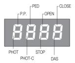
In the event of malfunctions, by pressing key + or - the status of all inputs (limit switches, control and safety) can be displayed. One segment of the display is linked to each input. In the event of failure it switches on according to the following scheme.
