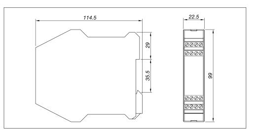
1. The enclosure of the Control Unit can be mounted in any position on a 35 mm IEC 60175 rail.
