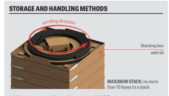
ASO edge material for self-assembly **MUST** be stored in a cool, dry environment away from sources of water or heavy contaminants. Before attempting to assemble contact edges the material should be checked thoroughly for moisture or contaminants and cleaned and dried appropriately.
