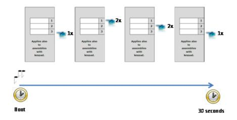
*Figure 3.7* Switching on Web Server Using Quick Dialling Buttons (Part Nos. 9137131E, 9137131CE, 9137131CKE)
