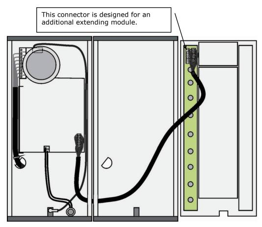
Figure 2.15 Connection of One-Row-Button Extending Modules
