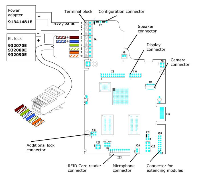
Figure 2.13 Description of 2N<sup>®</sup> Helios IP Connectors, PCB Version 535v5
