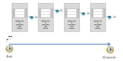
*Figure 3.8* Switching on Web Server Using Quick Dialling Buttons (Part Nos. 9137161E, 9137161CE, 9137161CE)
