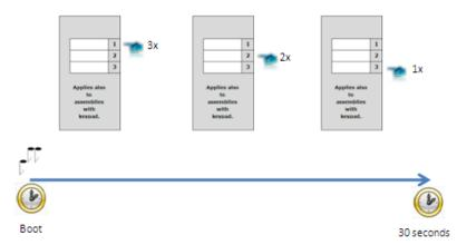
Figure 3.1 Switching to Default Network Parameters – Static IP Address (Part Nos. 9137131E, 9137131CE, 9137131CKE)
