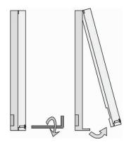
Figure 2.2 Cover Removing
