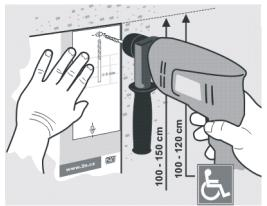
Figure 2.1 Hole Drilling
