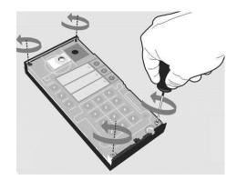
Figure 2.3 Plastic Cover Removing
