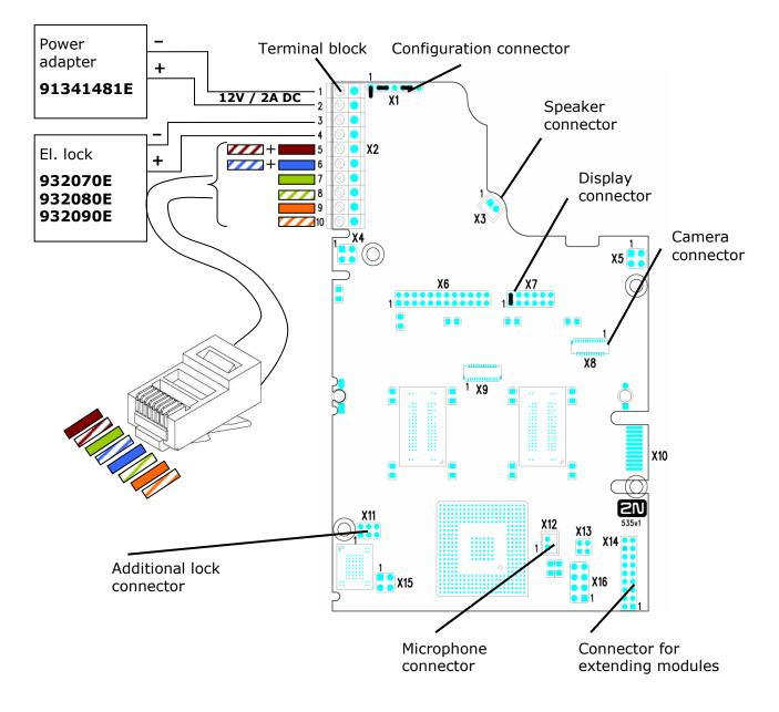
Figure 2.12 Description of 2N<sup>®</sup> Helios IP Connectors, PCB Versions 535v1, 535v2
