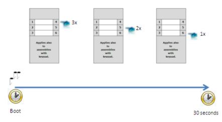
*Figure 3.2* Switching to Default Network Parameters – Static IP Address (Part Nos. 9137161E, 9137161CE, 9137161CKE)
