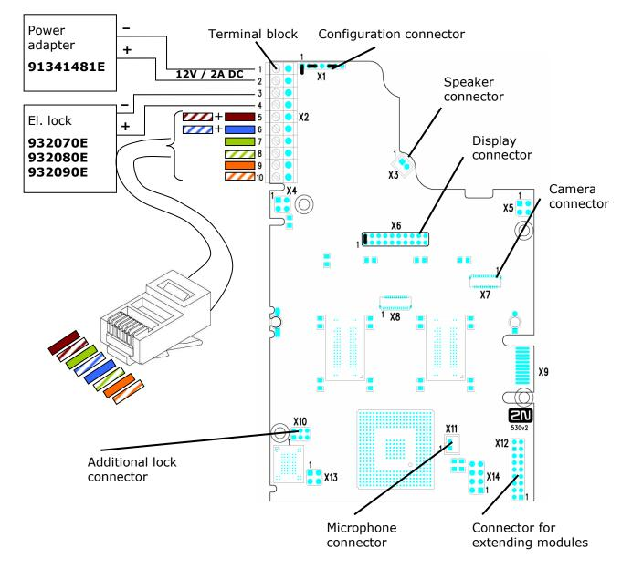
Figure 2.11 Description of 2N<sup>®</sup> Helios IP Connectors, PCB Version 530v2
