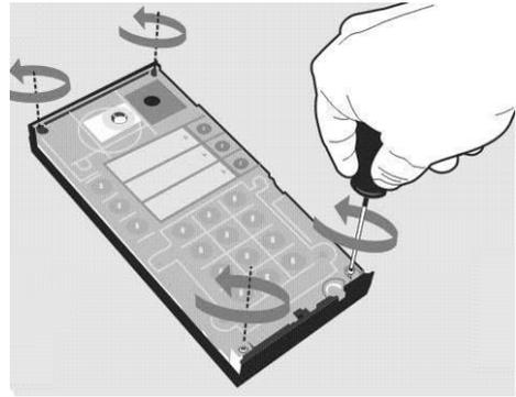
Figure 2.3 Plastic Cover Removing
