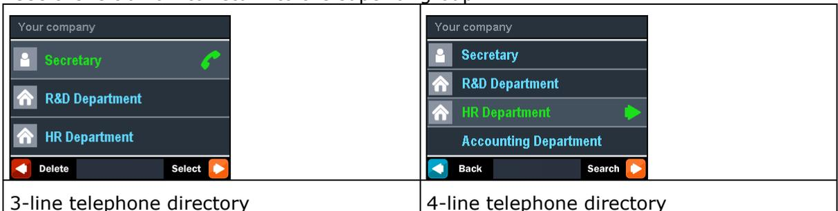
You can also use the telephone directory for retrieving contacts. Push the quick dialling button 6 to switch on the phone directory searching mode.
