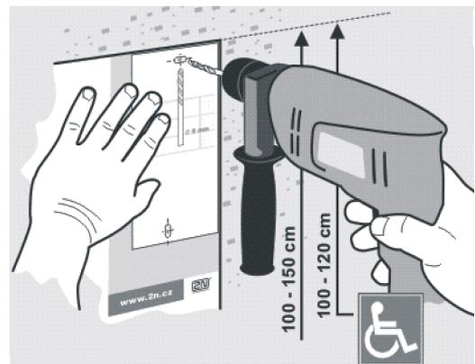
Figure 2.1 Hole Drilling
