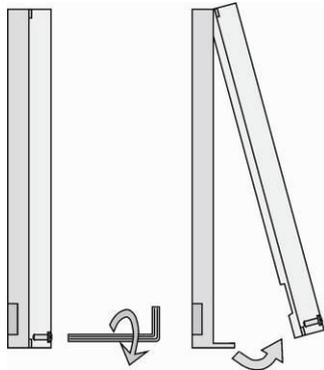
Figure 2.2 Cover Removing
